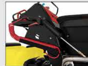
30-FT. EXTENDED HOSE LENGTH WITH HOSE TRAY
