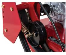
**SIMPLE DRIVE BELT MAINTENANCE** Drive belts can be changed quickly and easily, with no tools required. Deck belts can also be easily adjusted.
