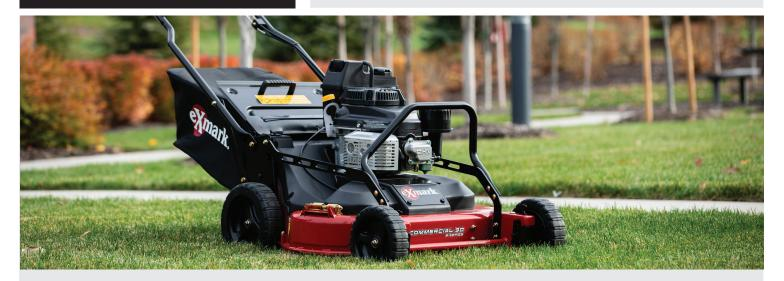
Don't let its size fool you. Our Commercial 30 mower is deceptively light and easy to maneuver. In fact, it feels and handles much like its Commercial 21 counterparts. The major difference: its 30-inch cut delivers up to a 40% increase in cutting efficiency compared to a standard 21-inch mower—without wearing out the machine or its operator.
