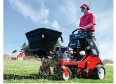
**SPREADER ATTACHMENT** With an 80 pound seed capacity, the spreader attachment enables landscape pros to offer over-seeding in conjunction with aeration programs. The versatility significantly increases the productivity in revenue potential of the machine. *(shown on 30" model)*
