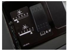
**ELECTRONIC DEPTH CONTROL** With the ability to easily set tine depth between 0.5" and 5", the Electronic Depth Control allows operators to maintain consistent core quality around a property.
